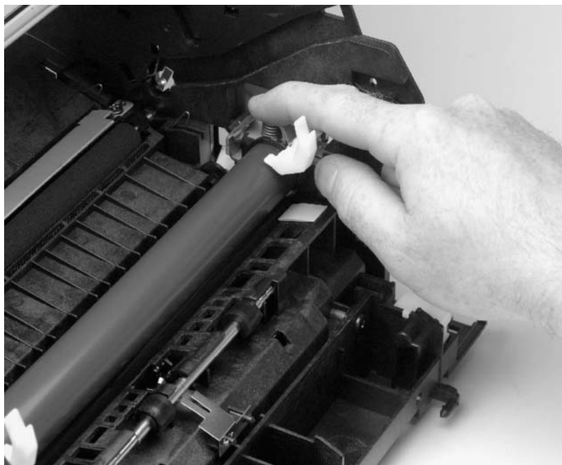
Figure 48. Fusing element metal clips reinstallation
